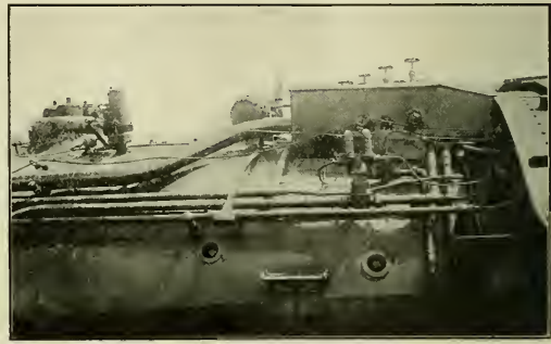
VIEW OF LOCOMOTIVE NO. 8000, SHOWING STEAM TURRET ON TOP OF BOILER IMMEDIATELY IN FRONT OF CAB
